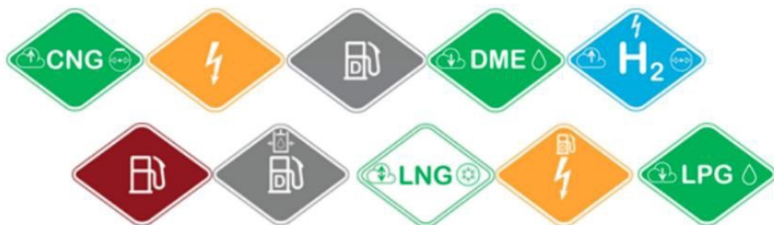
FIGURE 6. European marking system – alternative energy sources in vehicles. Source CTIF.
