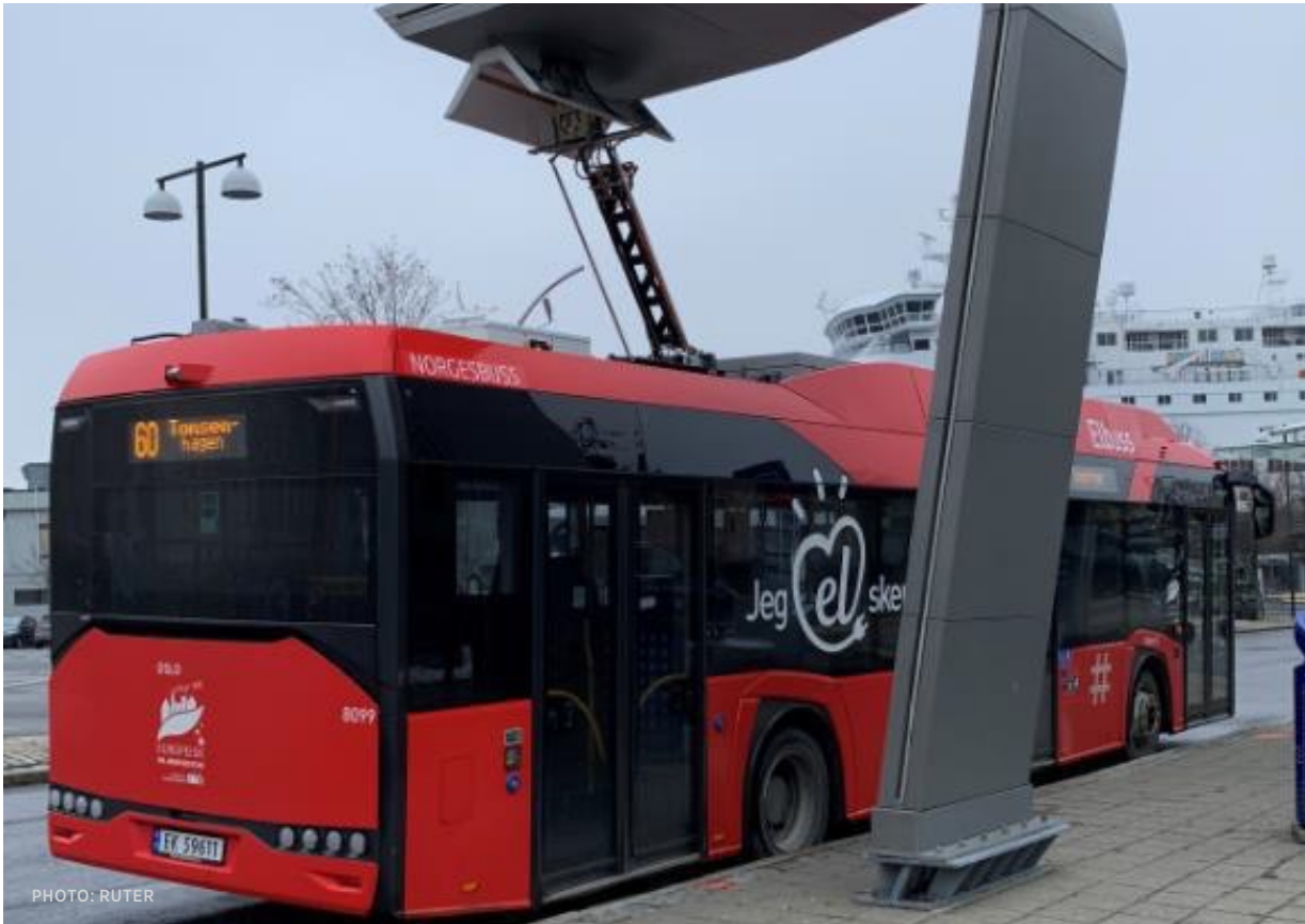
Charging of buses via a pantograph.
